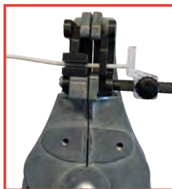
Transparent wire stop provides uniform stripping length
