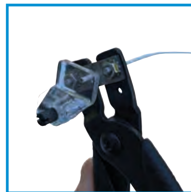
Adjustable wire stop for precision strip lengths
