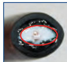
Bad oval dielectric
