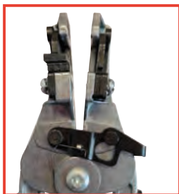
Short-stop latch protects wire strands by limiting the stripping stroke to 4 mm (5/32") and retains the slug until the wire is ready for termination
