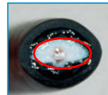
Bad oval dielectric
