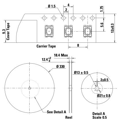
Note: Switches in reels of 2,900 pieces. Dimensions of reels according to EIA 481B. External diameter 330 mm.
