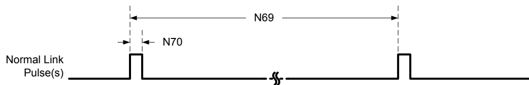
Figure 27-38. 10Base-TX Normal Link Pulse Timing
