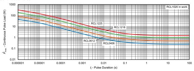
Maximum pulse load, continuous pulses; applicable if  $\bar{P} \leq P$  ( $\vartheta_{amb}$ ) and  $\hat{U} \leq \hat{U}_{max}$ ; for permissible resistance change equivalent to 8000 h operation
