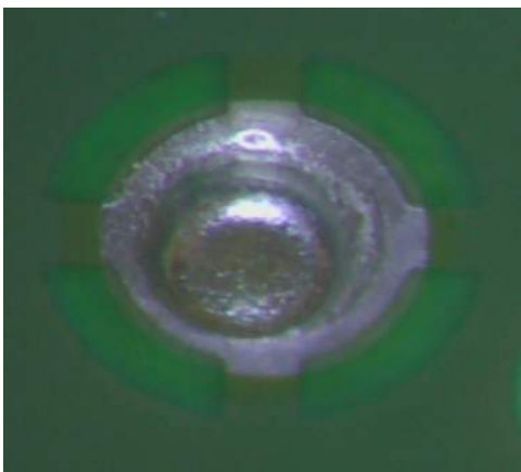
Soldered ground pin Lötstelle Masse-Pin
